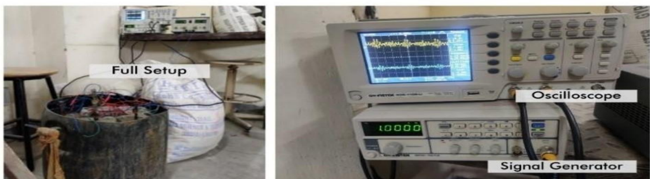
Figure 7: Test instruments equipment utilized in corrosion monitoring that transmits ultrasonic waves through concrete and steel, the frequency was likely selected.
