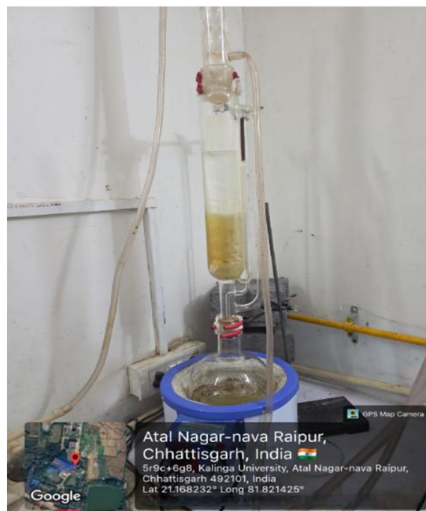
Figure 2: Soxhlet Extraction of Citrus limon Peel Using Ethanol
