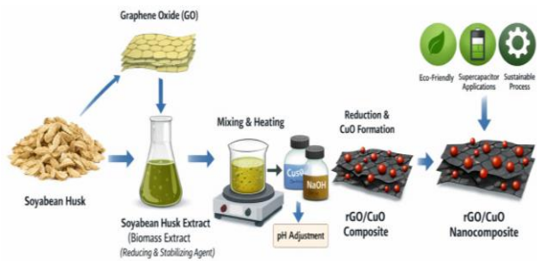
Figure 1. Soyabean husk-assisted green synthesis of rGO/CuO nanocomposite
