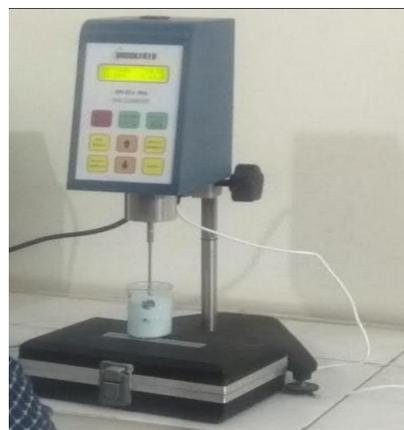
**Figure 2: viscosity of herbal shampoo by Brookfield viscometer.**
