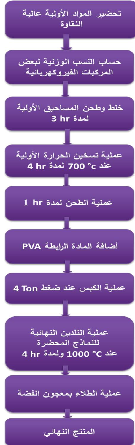
Figure 4: The stages of manufacturing ferroelectric models using the method of solid state interactions.
