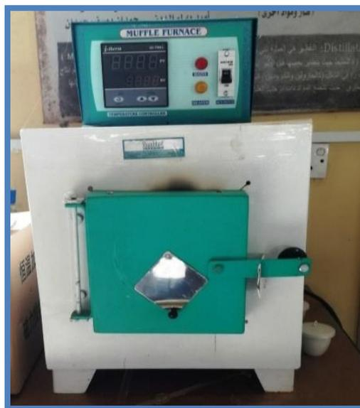
**Appearance 1: MUFFLE FURNACE electric oven, model SILMF-01**
