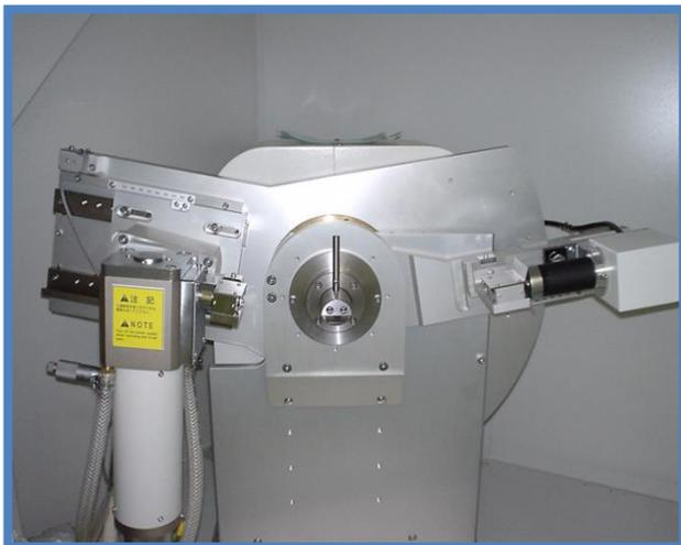
**Figure 5: X-ray diffraction apparatus**
